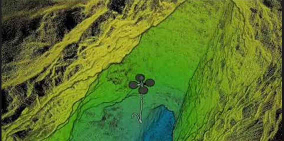
Screenshot showing the route the drone flew, and the data it collected, from the tallest stope of the trip.
