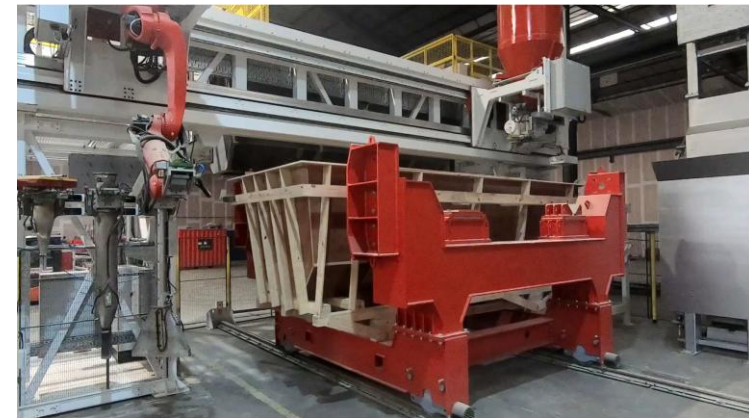
Tundish DryVibratable Robot at our robotics centre, Ghlin, prior to transportation and installation to Nucor West Virginia
